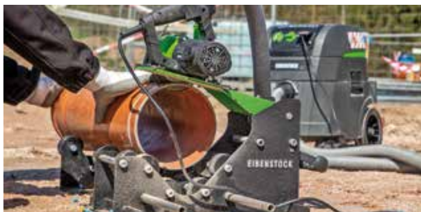
Cutting and chamfering in one step
